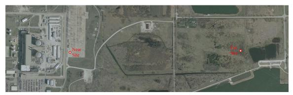
Figure 1: Arial photograph of the Braidwood Nuclear Power Station showing the locations of the near and far investigative bore holes. The bore holes were located at the proposed shaft sites.
